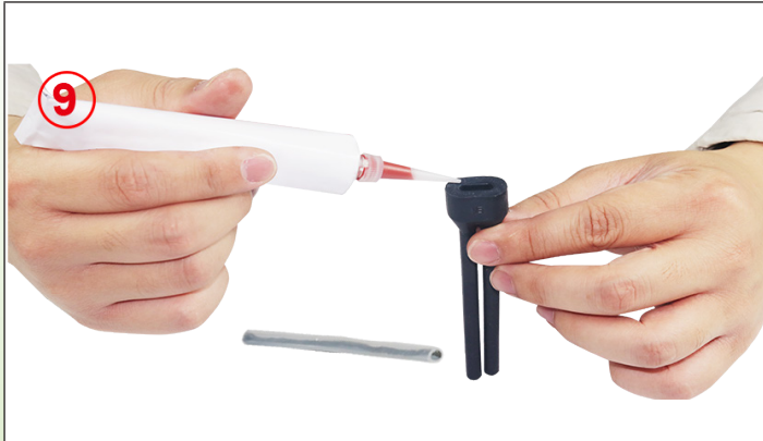
9: Pour RTV silicone inside the main hole of the two holes silicone boot.
